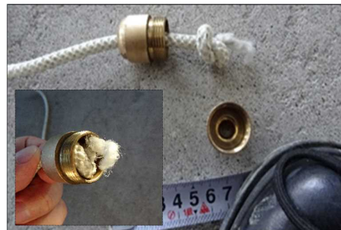
Figure 4: Fractured at a knot in the sleeve
