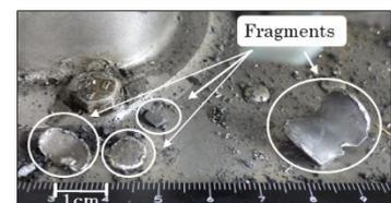
Figure 2d Fragments of (typical) blades penetrated the compressor case
