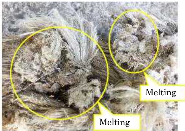
Photo 2.9-3 Traces of Melting
