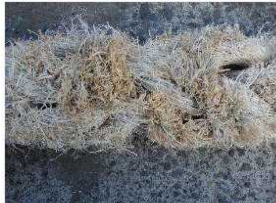
Photo 2.9-2 Inability to Distinguish Strand Shapes
