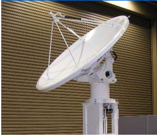
Multi-Parameter Weather Radar
