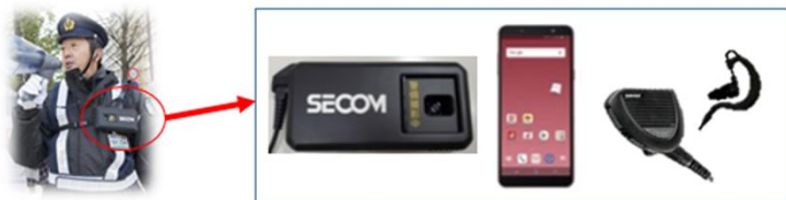
Smart Phone+Special Case+Special Speaker Microphone/Earphone
