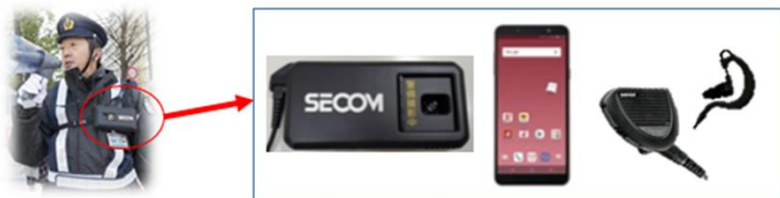
Smart Phone+Special Case+Special Speaker Microphone/Earphone
