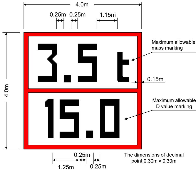
Figure 2.9.3 Example of maximum allowable mass marking and maximum allowable D value marking
