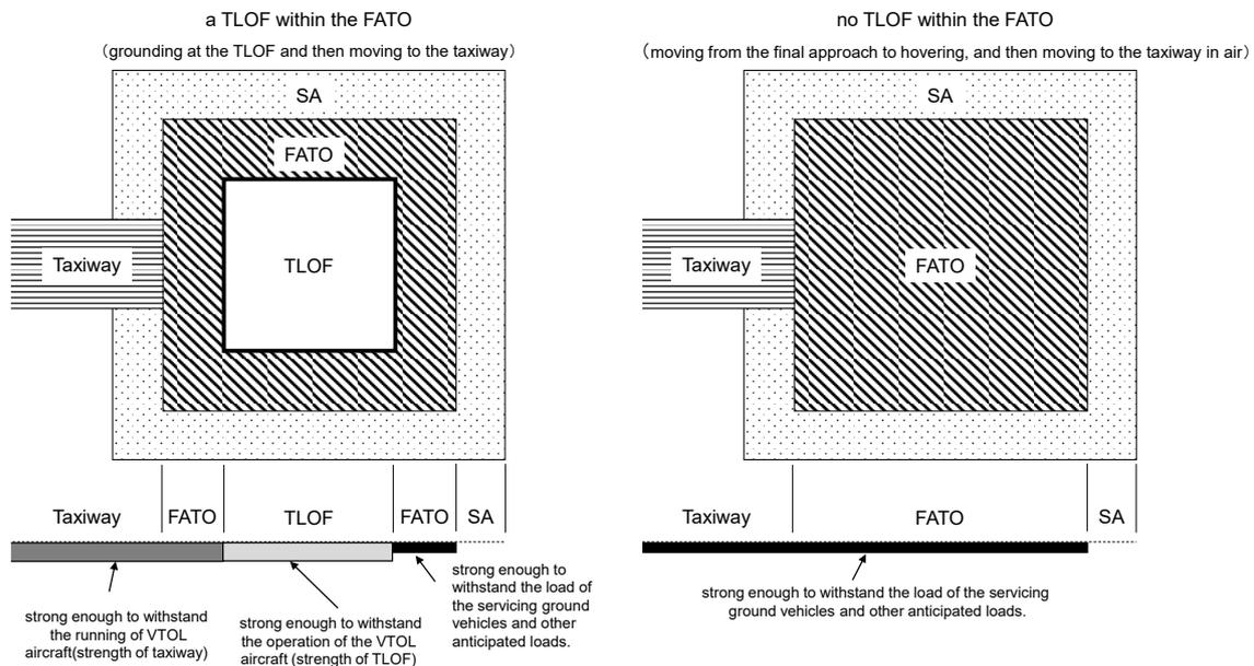
Figure 2.1.3 Example of strength level in the case of a paved FATO
