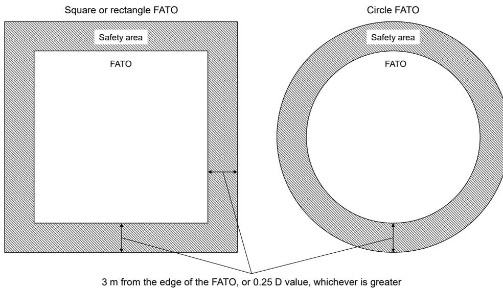
Figure 2.2.1 Example of size and shape of a SA
