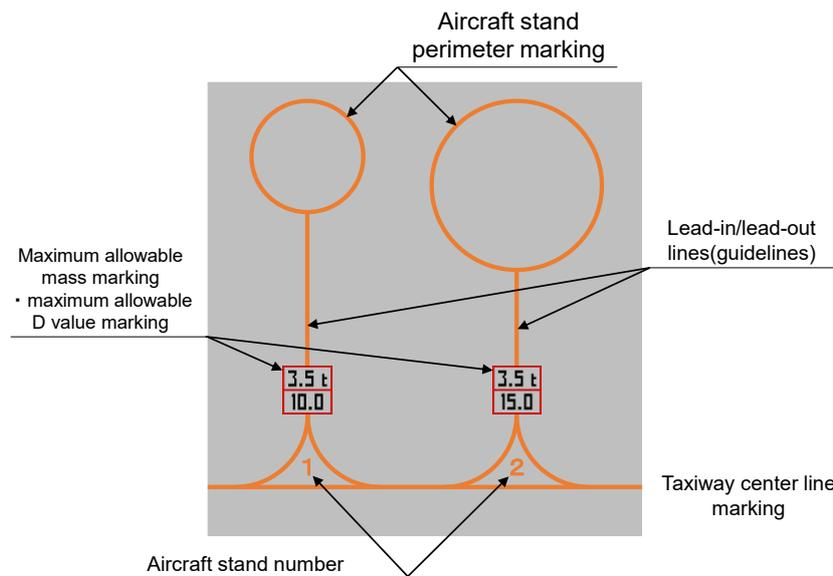
Figure 2.9.6 Example of apron markings indicating D value limitations
