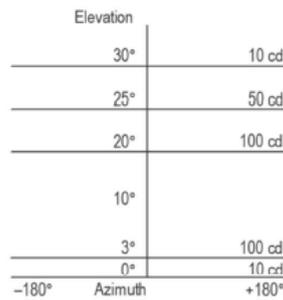
Figure 2.10.3 FATO perimeter light isocandela diagram
