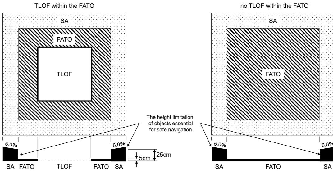
Figure 2.1.1 Height limitation of objects essential for safe navigation within FATO and SA (in the case of a rectangular FATO)
