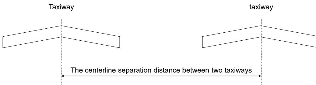
Figure 2.5.1 Centerline separation distance between two taxiways
