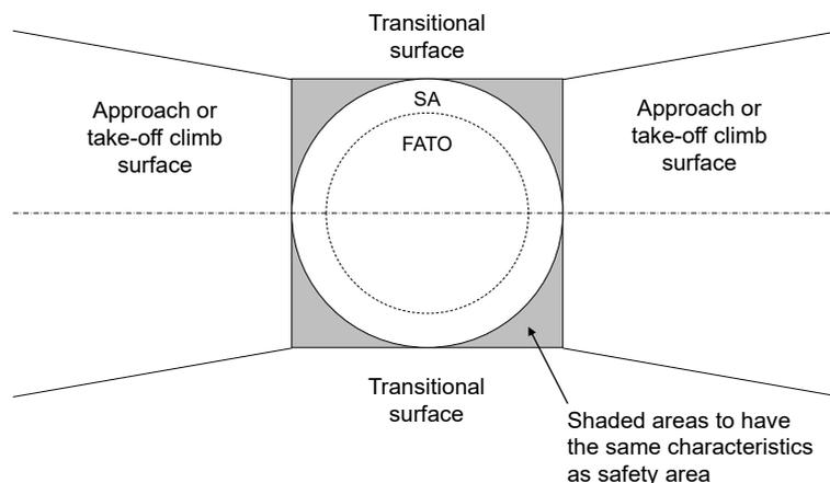
Figure 3.1.3 Illustration of obstacle limitation surfaces for a circle shaped FATO
