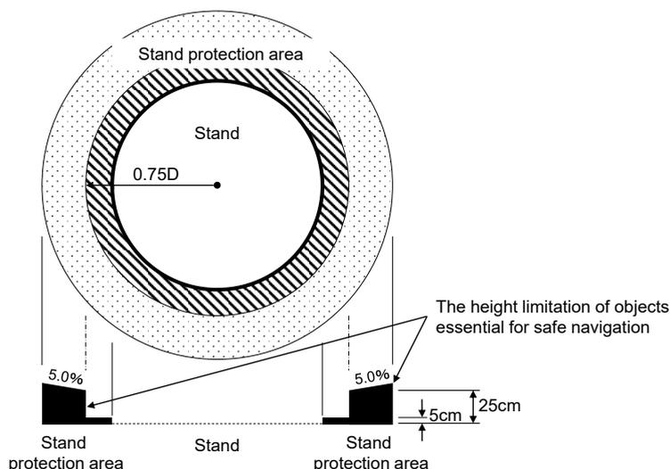
Figure 2.8.1 Height limitation of objects essential for safe navigation within a stand protection area
