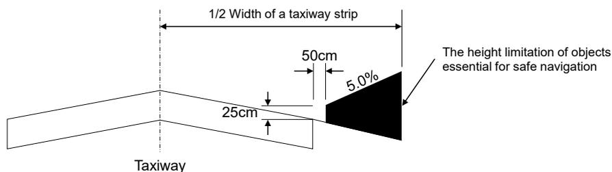
Figure 2.6.1 Height limitation of objects essential for safe navigation within a taxiway strip
