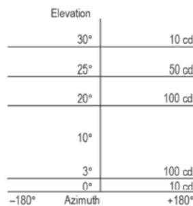
Figure 2.10.6 Aiming point lights light isocandela diagram
