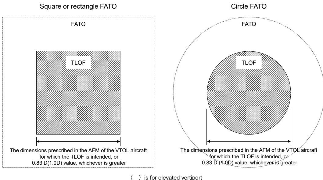
Figure 2.4.1 Example of size and shape of a TLOF
