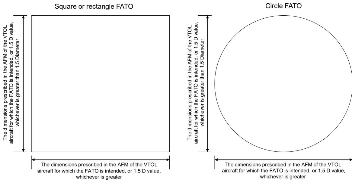
Figure 2.1.2 Example of size and shape of a FATO
