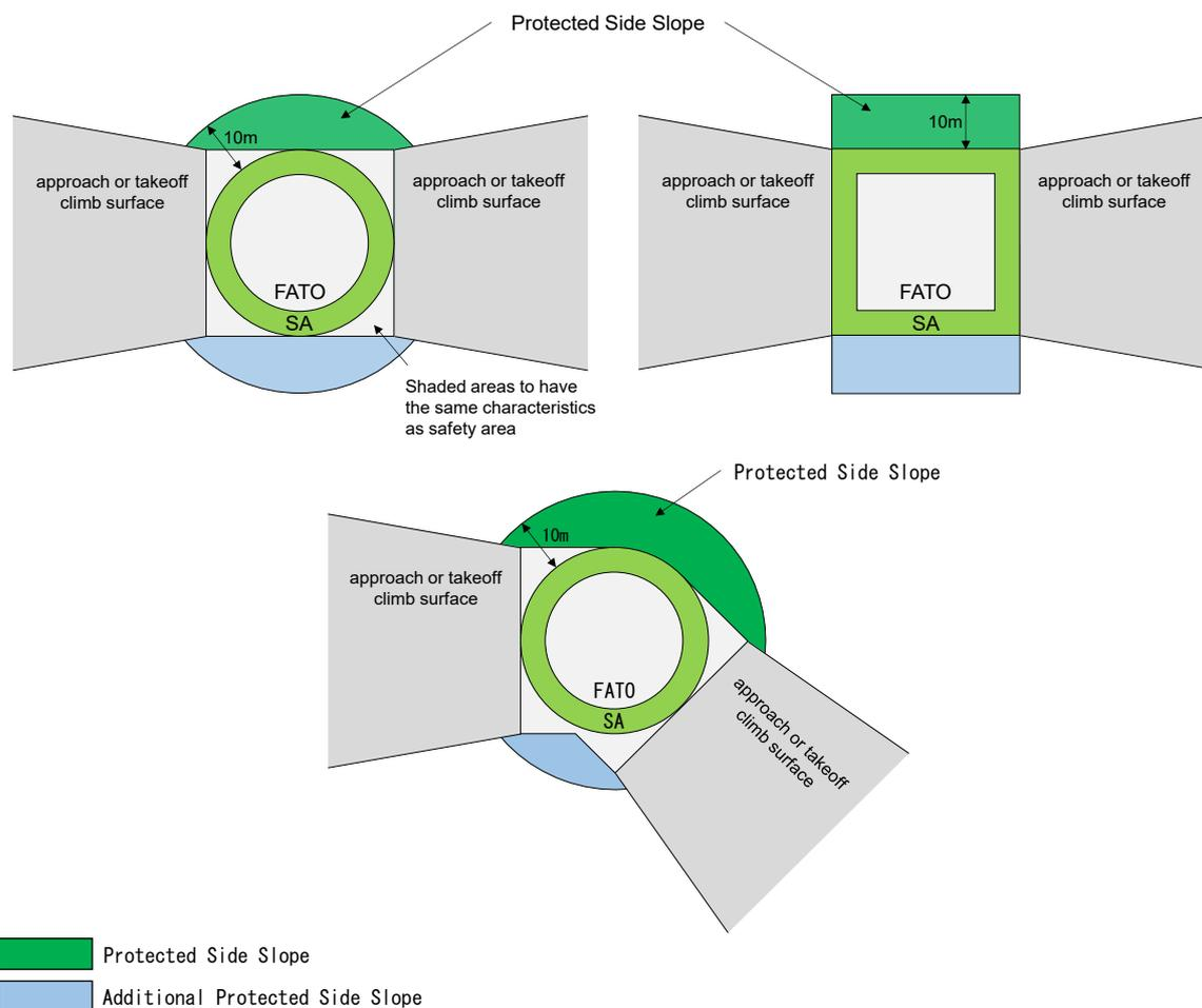
Figure 2.3.1 Example of Protected Side Slope
