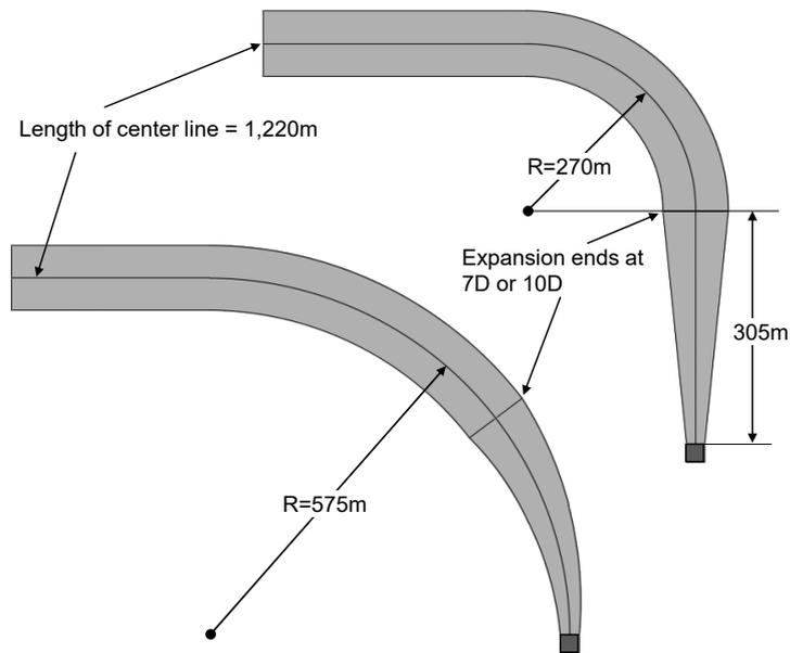
Figure 3.2.1 Example of an approach or takeoff climb surface with a curved portion
