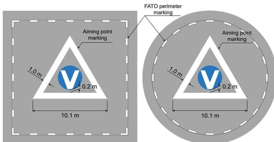
Figure 2.9.2 Aiming point marking
