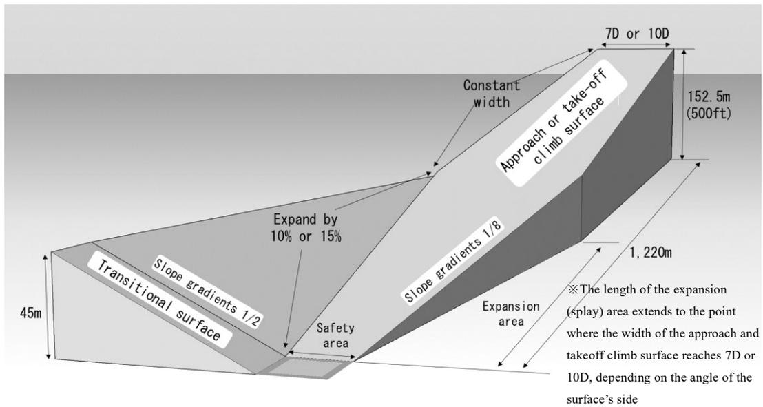
(a) Isometric view of approach or takeoff climb surface and transitional surface
