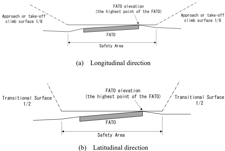
Figure 3.1.2 Illustration of the minimum heights of approach surface, takeoff climb surface and transitional surface
