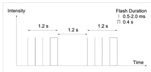
Figure 2.10.1 Vertiport beacon flash characteristics
