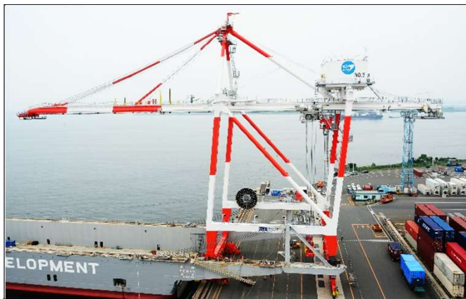
Introduction of inverter-controlled gantry cranes (New Unit 3 installed at T1 Pier)
