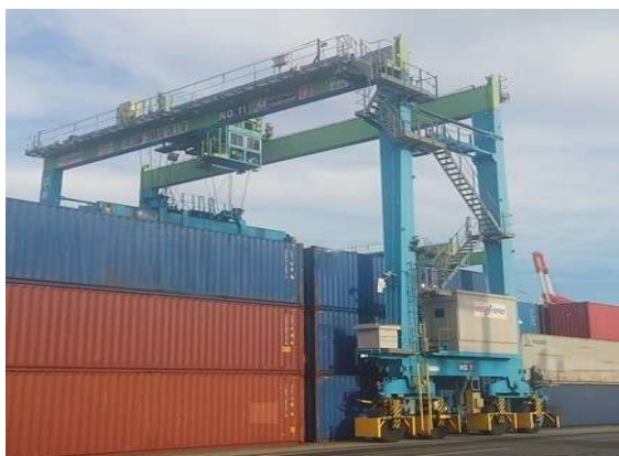
Container handling operations using hybrid RTG
