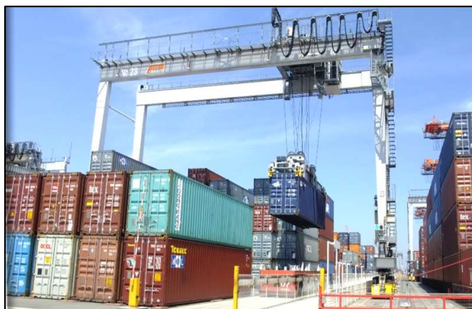
Automated container operations ARTGs and AGVs (Idling-free & Lights-out operations)
