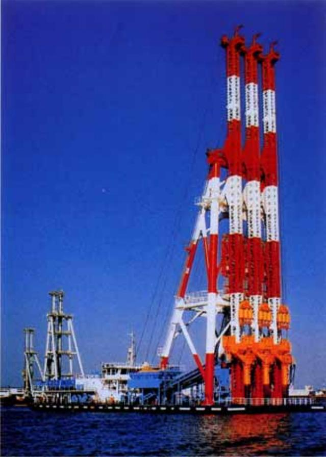
A large, specialized vessel used for sand compaction. It features a prominent red and white structure with multiple vertical columns. The vessel is shown on the water, with another smaller vessel visible in the background. |
