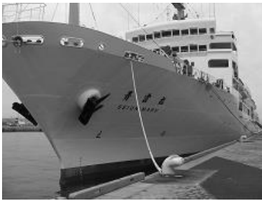
写真11 Forward Breast Line
