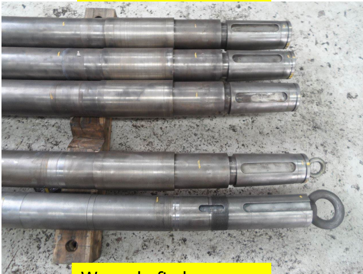
Worn shaft sleeve
