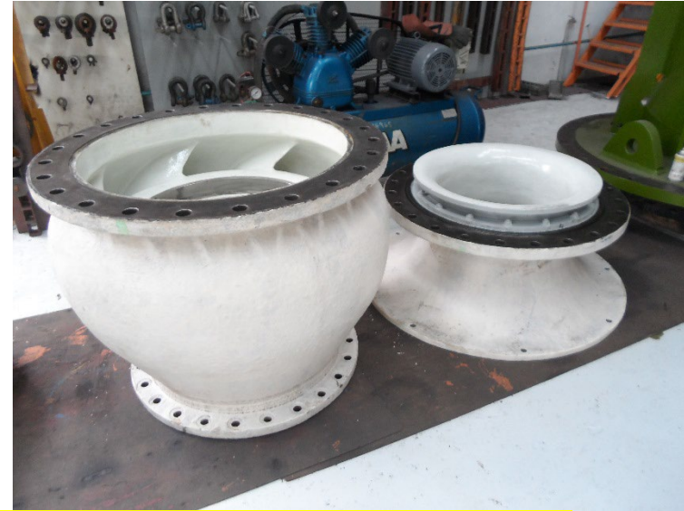
Repaired by coating on Vertical Turbine Pump parts
