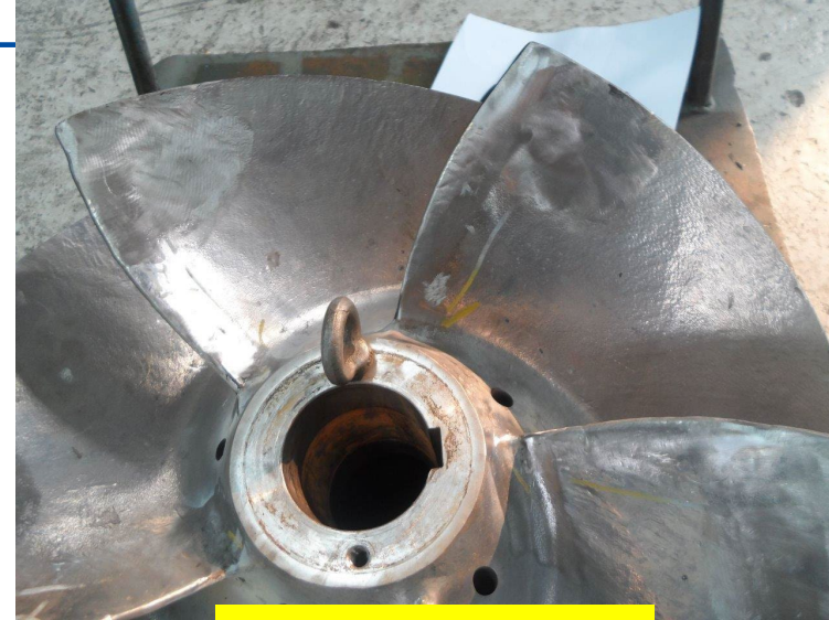
After welding repair
