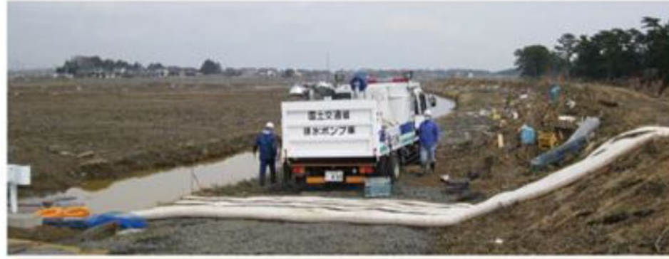
Example of Working situation of Truck Pump mounting Super Light Pump for Disaster
