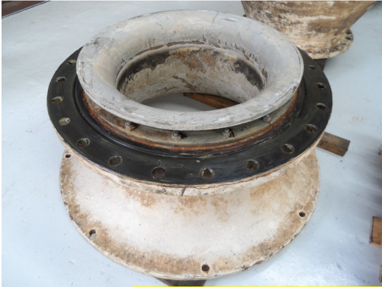
Repaired by coating on Vertical Turbine Pump parts
