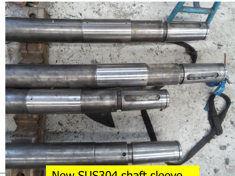
New SUS304 shaft sleeve
