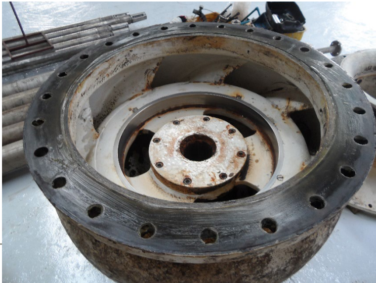
Repaired by coating on Vertical Turbine Pump parts
