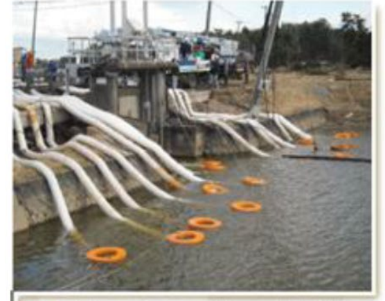
Example of Working situation of Truck Pump mounting Super Light Pump for Disaster
