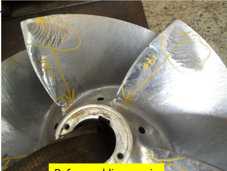
Before welding repair
