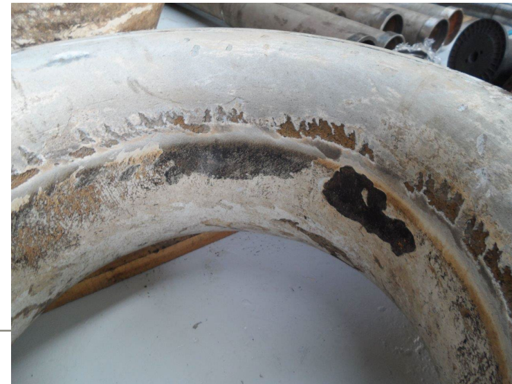
Repaired by coating on Vertical Turbine Pump parts
