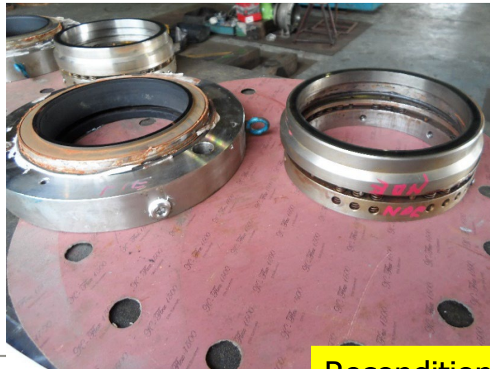
Reconditioning of Mechanical Seal
