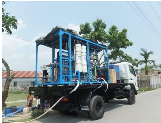
Truck-mounted Treatment Unit (RO Filter)
