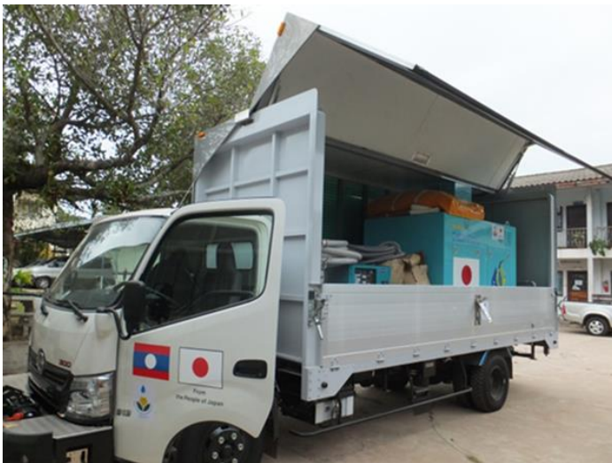
Truck-mounted Treatment Unit (Sand Filter)
