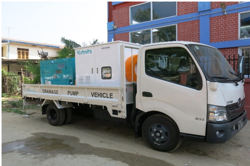
Completed Drainage Pump Vehicle
