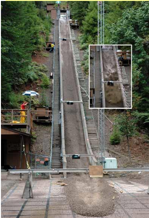
←USGSの実験水路(長さ95m, 勾配31度) https://pubs.usgs.gov/of/2007/1315/
