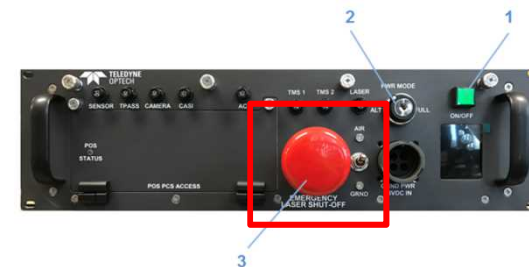
1 - ON/OFF main power button, 2 - Laser key switch (PWR MODE), 3 - Emergency laser shut-off button (kill switch)
