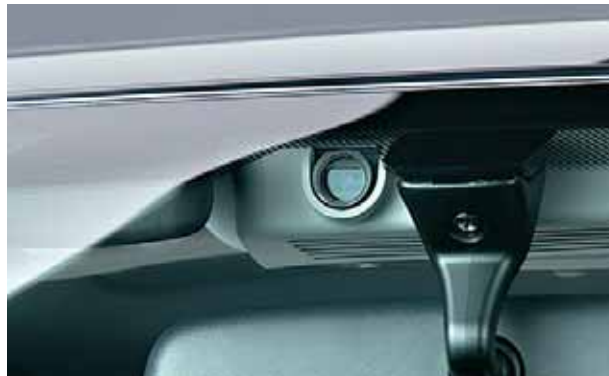
Lane departure warning and camera to support lane keeping
