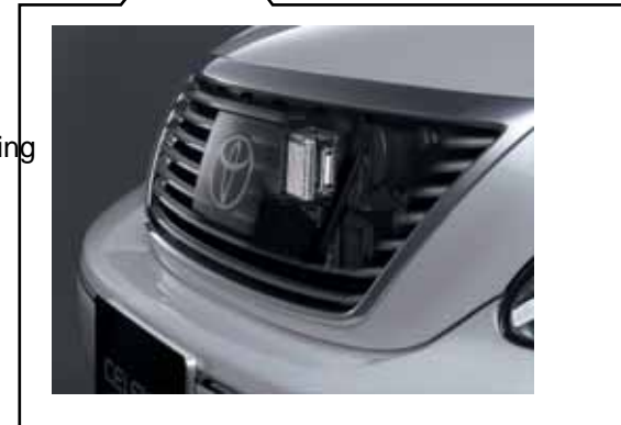
Example of technology for braking control to reduce collision damage
