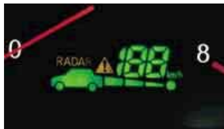
Example of technology to automatically adjust following distance using ACC
