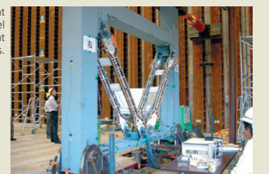
A model experiment using a 1/6-scale model of buckling restraint braces.
