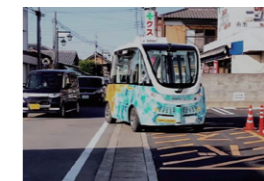
Self-driving bus operation in Sakaimachi, Ibaraki Prefecture (Increase the number of bus stops and waiting areas to eliminate the delay of following vehicles)
