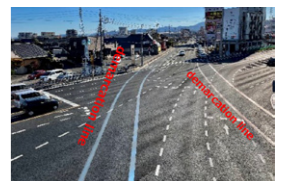
Verification of support measures at complex intersections (image) (Maintenance of demarcation lines to be detected by in-vehicle sensors)
