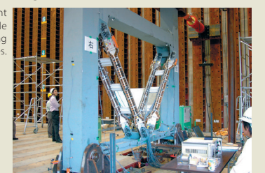
A model experiment using a 1/6-scale model of buckling restraint braces.
