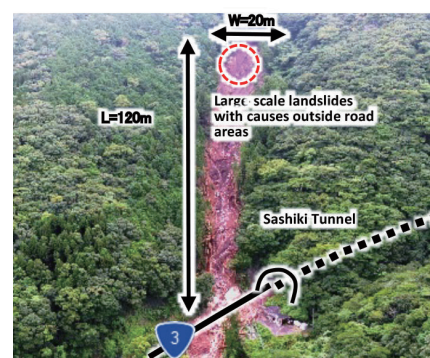
Large-scale landslide from a slope adjacent to the road area National Route 3 Heavy rain in July, 2020
