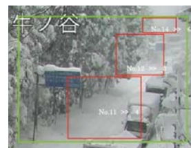
Automatic traffic obstacle detection system
