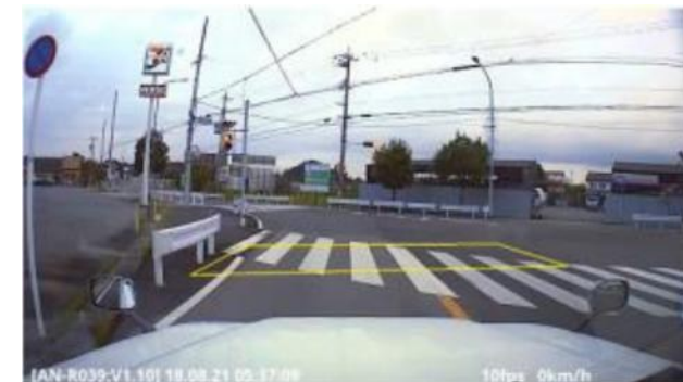
Lane line wear judgement using images obtained from drive recorder
