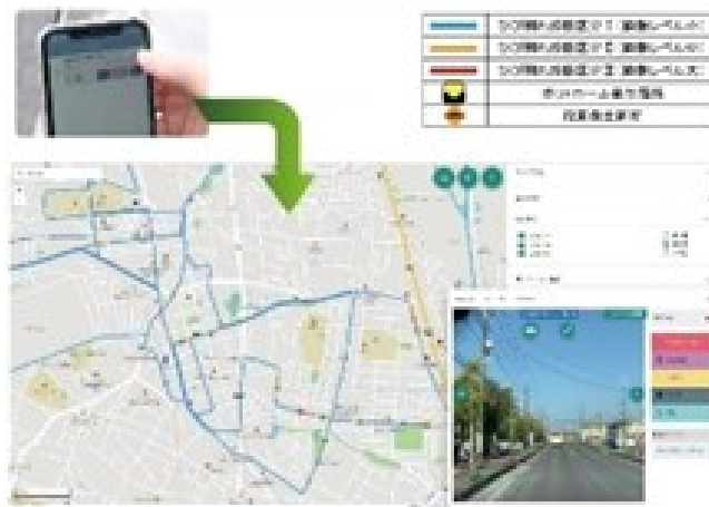
Pavement condition measurement using images and acceleration obtained by smartphone
