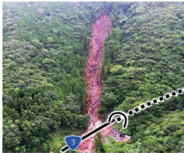
Massive collapse from the top of the slope Heavy rain in July 2020 (National highway 3, Ashikitamachi Kumamoto Prefecture)
