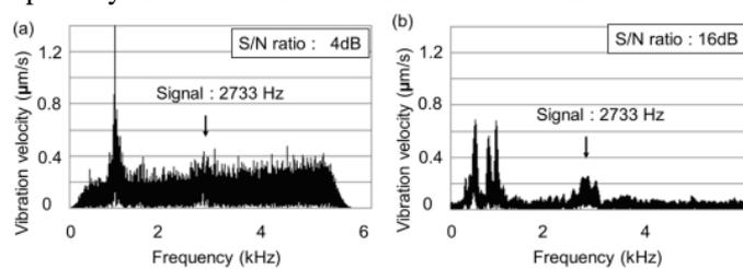
Fig.1. Vibration velocity spectra on the damaged part. (a) chirp wave, (b) Tone burst wave with time gate.
