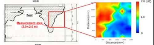
Fig.4. Experimental results. (a) Hammer method (slash part :float), (b) Non contact acoustic inspection method using vibration energy ratio.
