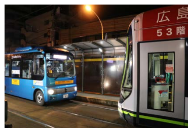
Fig.5 World's first pilot test of connected system of autonomous bus and LRT
