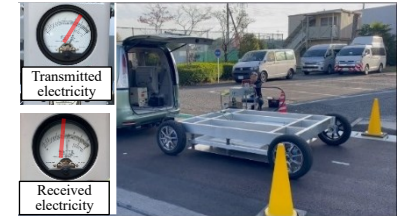
Fig. 3 Dynamic wireless power transfer experiment
