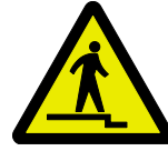
下り段差注意 Caution, uneven access/down
