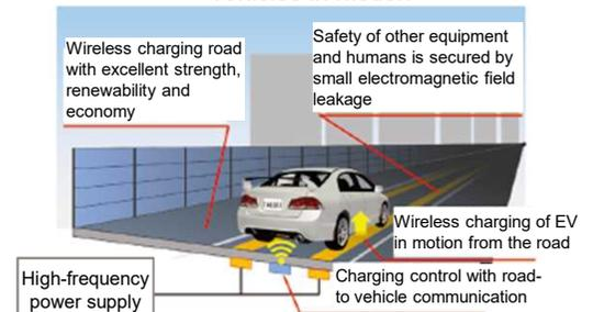
Wireless charging of vehicles in motion is expected to provide a solution to issues such as cruising distance
