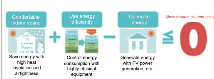
Net Zero Energy House (ZEH) refers to a house that cuts primary energy consumption by 20% or more from the energy efficiency standards with energy saving measures and reduces primary energy consumption by 100% or more with the introduction of renewable energy and other means.
