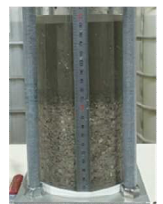
No.1(Bor-3,4) 判定B 浸透層厚12mm
