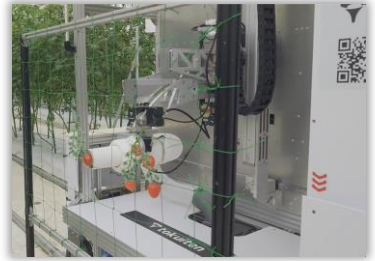
Automated suction-type harvesting robot for mini tomatoes
