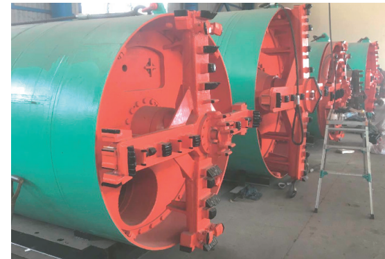
High-density slurry type pipe jacking machine in Vietnam
