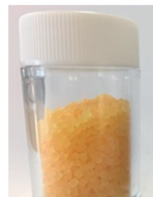
Asphalt modifier material for porous asphalt pavement -TPS
